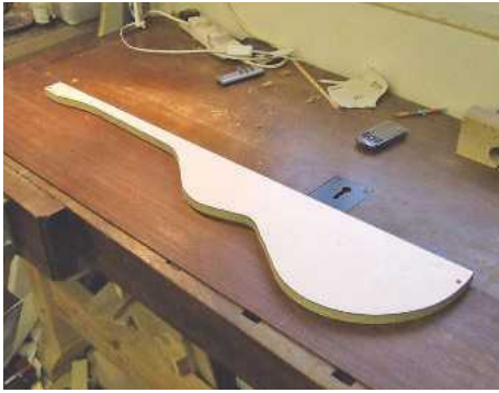
▲ Pic.1 Phil used a half template for the top and bottom of the guitar
